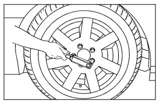
Loosen the wheel nuts, but do not remove them yet, using the wheel wrench. Turn the handle about 180 degrees, then flip the handle back to the starting position. This avoids taking the wrench off the lug nut for each turn.
